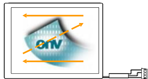
Fig. 2 Reverse scan (Pin19 = High)
