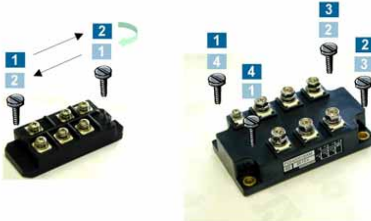
Sequence of tightening screws
